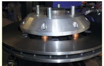
At this stage you cannot fit the rotor/bell assembly to the upright, but it is necessary to position the disc in its ideal location and slide caliper/pad assembly onto the rotor to check all clearances.
